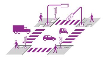
It is suggested that pedestrian crossings be at sidewalk or road level (with ramps of at least 0.8 m of width at both ends and a maximum slope of 8%), that intersections create 90° degree angles, and that they have appropriate horizontal markings. It is also recommended to reduce the number of roads that share the intersection, and the allowed vehicle maneuvers.
