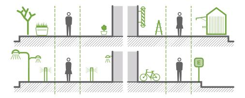
The services section of the sidewalk is a space with the ability to host several types of infrastructure at the same time. The variety and spacing between the components depends on the urban context and the road's service level. However, it is suggested that the following be installed:
