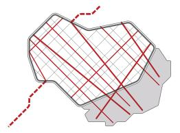
The borders of the sustainable urban community must have an intersection at least at every 250 meters within its perimeter, which represents half the walkable distance between two intersections. Not all roads must necessarily be built for vehicular traffic. They can also be wide pedestrian and cycling paths.
