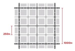
To ensure a high degree of connectivity, compliance with a minimum index of 1.4 is recommended 1. This index is calculated by dividing the number of segments (road links between intersections) by the number of nodes (intersections) within the surface of the neighborhood. A score of 1.4 implies more direct connections to travel between two points, as on average, there will be more paths available from each intersection.
