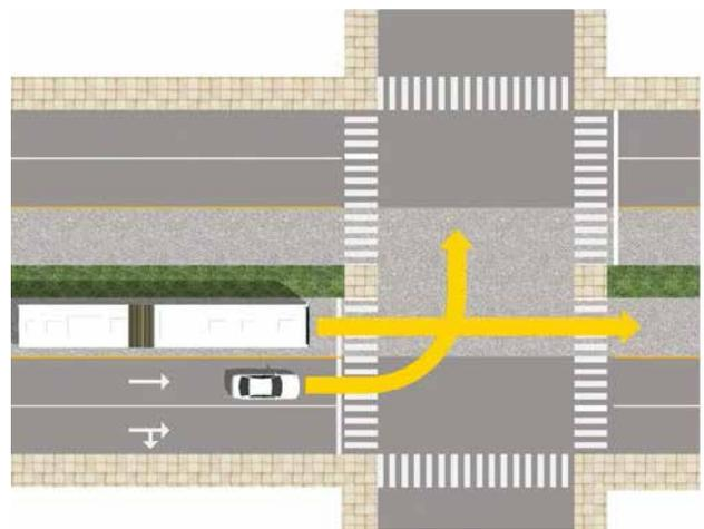
**Figure 16** Center BRT lanes with mid-block crossing on a urban arterial (EMBARQ, 2012)
